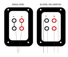
Totem speakers feature binding post terminals that accommodate 5 methods of connection: bare wire wrapped around the post, wire through the hole of the post, pin connectors through the posts, banana plugs, and spade lugs. A spade lug size of 8.1mm / 5/16" to 9 mm / 3/8" is required for proper fit. We recommend the WBT 0681 spade for its quality and fit but any spade in the size range can be used.
