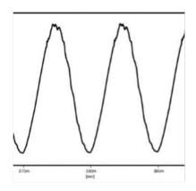
The most common source of speaker damage results from amplifier distortion. Your amplifier may run out of clean power upon listening at loud levels. A direct consequence of such an overuse is distorted power, producing a greater quantity of distortion than its rated output power. This provides a threat of damage to any loudspeaker.
