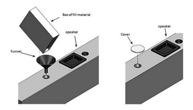
**Note:** Always remember to apply the plastic adhesive stopper to seal the cavity. To prevent damage, the speakers, should never be transported with mass inside. The cavity must be emptied prior to transport by using a shop vac and sealed thereafter using a sturdy tape to avoid any loose sand from migrating. Totem recommends the use of clean dry sand, silica sand, dry particulate matter, or non-odor kitty litter.
